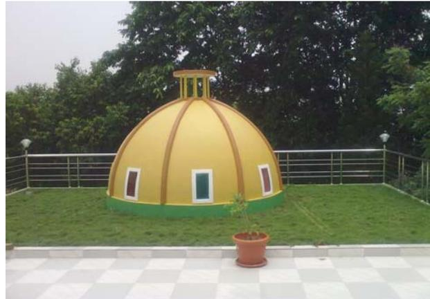
Dome with NAC – lawn is grown on the slab in order to induce hostile conditions of weathering.
