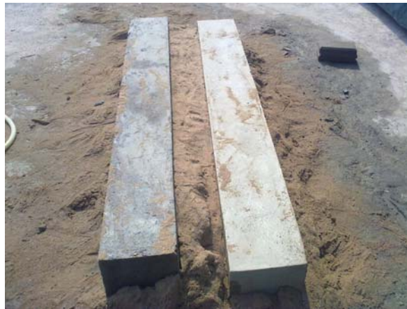
RCC beams: with OPC concrete (left) and NA-concrete (right)
