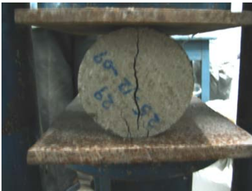
Split cylinder strength test on NAC cylinder
