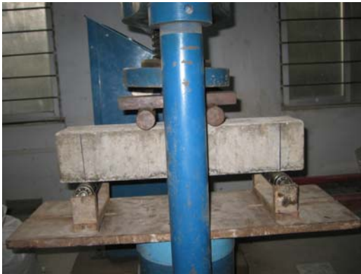
Testing on NAC beam-specimen
