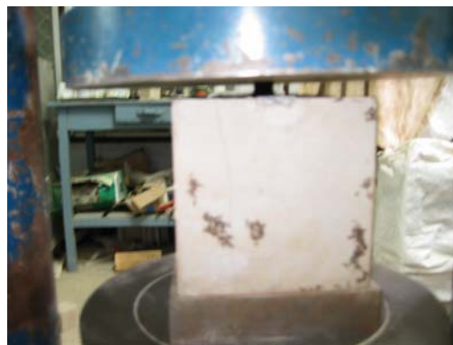
Study of bond strength on NAC specimen
