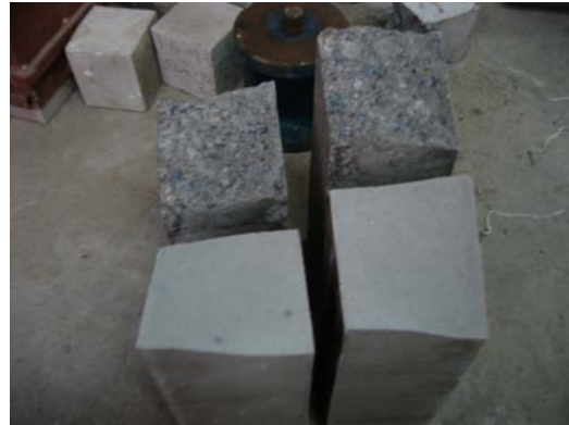
Phase of concrete after breaking the beams
