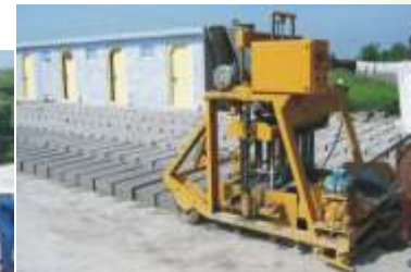
Production in Egg-laying machine (Vibro -compactor)
