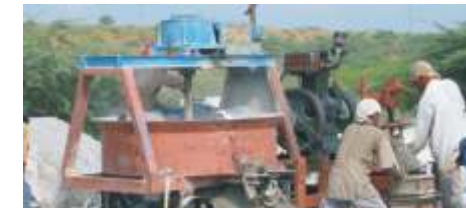
Production in Vibro - Table attached to roller mixer with single engine
