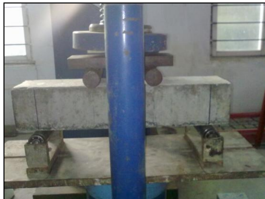
NAC beam positioned for flexural strength (MOR)
