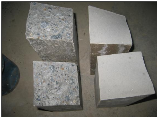
Beams tested for flexural strength: control Vs NAC concrete
