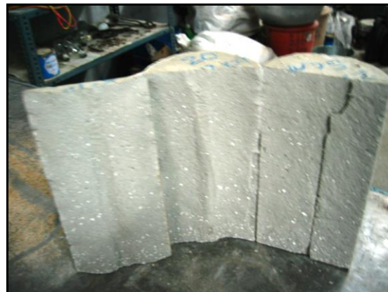
NAC cylinder after Split tensile strength
